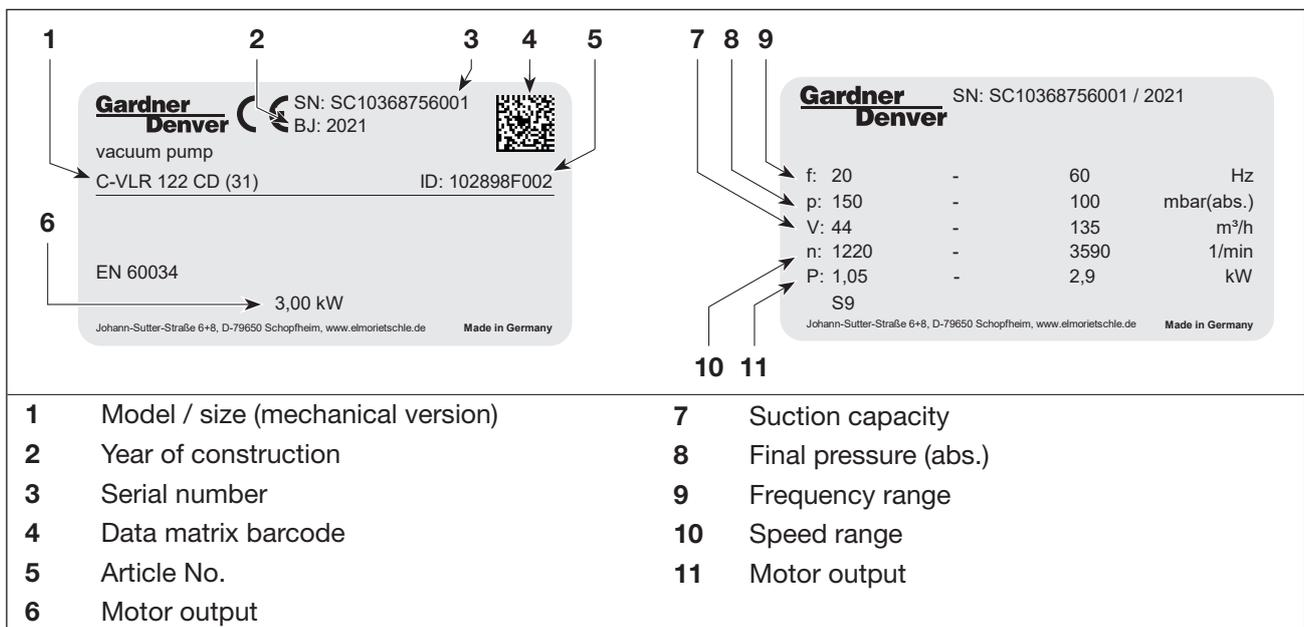
Fig. 6 Data plates for machines with frequency converter
