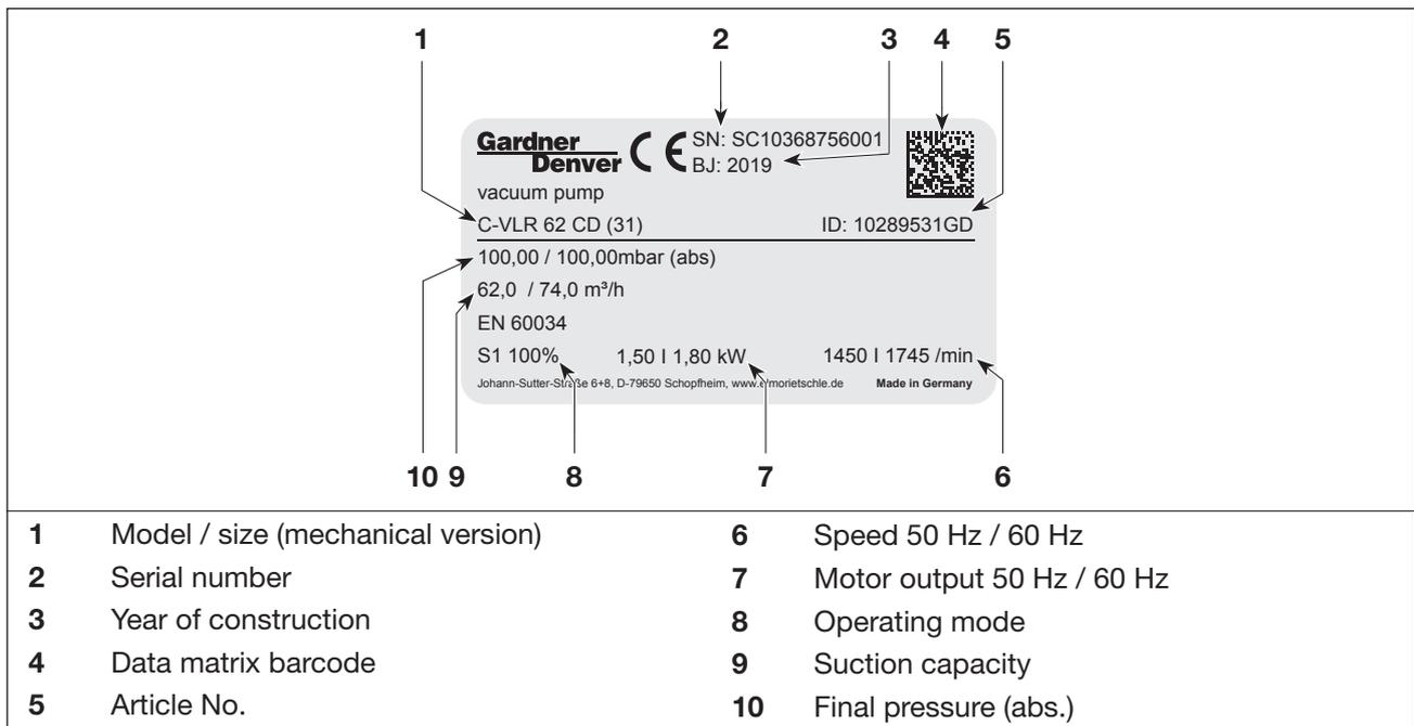
Fig. 5 Data plate for machines without frequency converter
