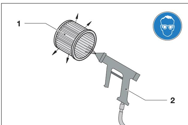
Fig. 6 Purging filter cartridge
