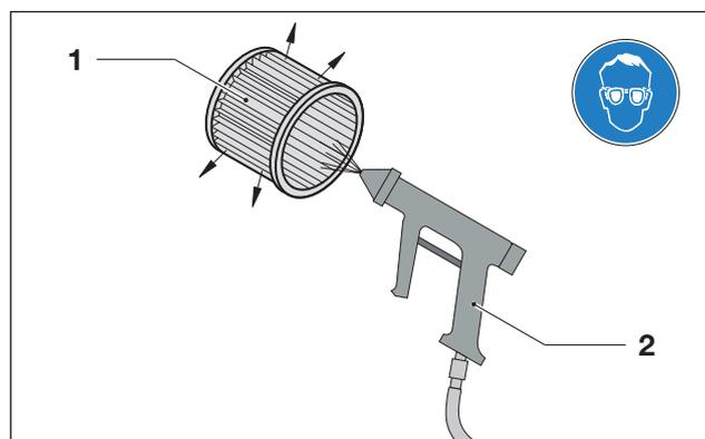
Blow off the filter cartridge (1) using compressed air (2).
